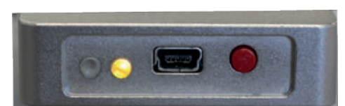
Operator/Data Transfer end of the PowerMAP® II. Different modes (Stop, Run, Pause) are indicated by the color of the LED.
