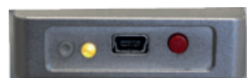
Operator/Data Transfer end of the PowerMAP® II. Different modes (Stop, Run, Pause) are indicated by the color of the LED.
