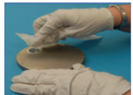
3) Use of EIT Instrument Wipe in a circular motion while using different parts of the nonabrasive wipe
