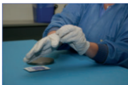
2) Using gloves to prevent transfer of finger oils
