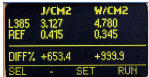
Reference Mode allows user to compare present reading with previously recorded values.
