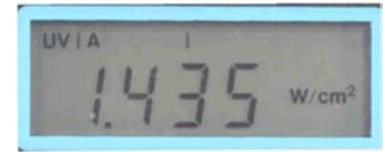
Display showing a "UVA" MicroCure and irradiance values.
